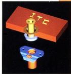
INTERNALLY THREADED FASTENER WITH TAPERED SLEEVE BOLT AND INTERNAL DETENT RING.
