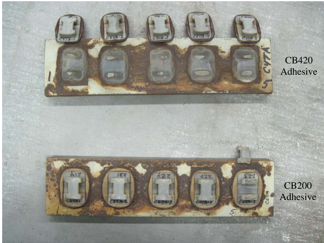
PHOTO 9 – CB9205VF STRAP FASTENER LOOPS BONDED WITH CB200 ADHESIVE AFTER ENVIRONMENTAL CONDITIONING AND TESTING
