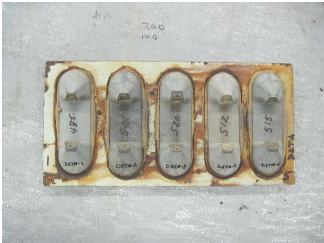
PHOTO 9 – CB9205VF STRAP FASTENER LOOPS BONDED WITH CB200 ADHESIVE AFTER ENVIRONMENTAL CONDITIONING AND TESTING
